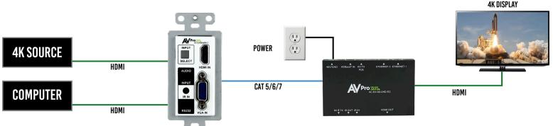
THE LITTLE GIANT WALL PLATE IS THE ONLY HDMI/VGA TRANSMITTER IN THE WORLD THAT IS ABLE TO FIT INTO A SINGLE GANG Wall mud ring. And power is never a question. The little giant is able to get power from the reciver end.
