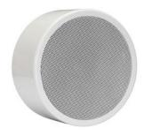
The EN-SM6T10-W is a surface mounted speaker made of powder coated steel (RAL 9010 equivalent), equipped with a high efficiency full range speaker and a multi tap 100 volt transformer, all certified according EN 54-24. The unit is equipped with a ceramic speaker line connector block and thermal fuse.
