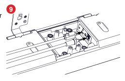
10. Rotate the bar up to rest against the underside of the bracket. Use two hands in the middle of the bar to rotate it. Don't use a twisting motion or rotate from one side only. Route cables through the side cutouts in the bracket.
