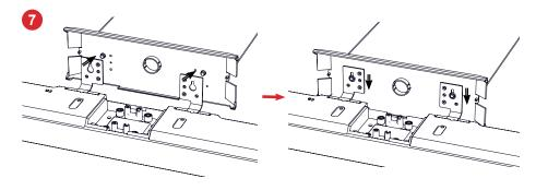
Secure the bar to the bracket by inserting 8. the screws (reserved from the table stand removal) through the hinge plates and fully threading them into the bracket (2 screws per hinge).
