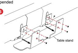
Open the hinges and hang the bar on the knobs on the underside of the bracket. The bar will be fully supported by the cables at this point.
