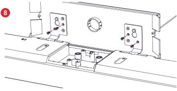
Connect the power / USB / audio cables. Screw the power and USB cables into the port jacks to secure them. Refer to the installation manual for complete bar instructions. (bia.mp/ABC-VBC\_manual)
